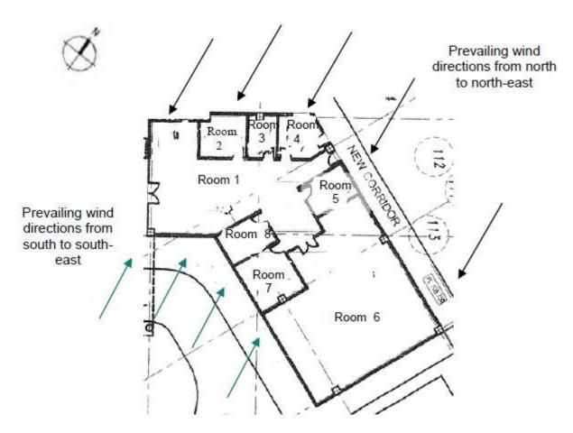
Building layout shows not all rooms with window openings facing the north and south directions. Room 2 to Room 5, Room 7 and Room 8 would only have prevailing wind in one direction. Only Room 1 and 6 can be considered meeting the requirement.
