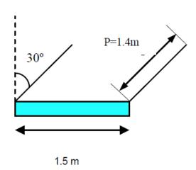
Check: To determine if the sun shading provisions (i.e. vertical projection (P)) meet the minimum 30% shading.
