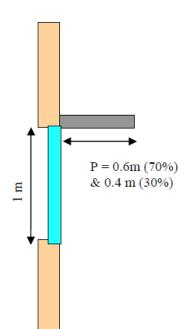
Check: To determine if the sun shading provisions (i.e. horizontal projection (P)) meet the minimum 30% shading.
